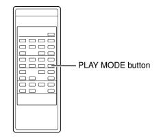
**1** While stopped, press the PLAY MODE button on the remote control unit repeatedly.
